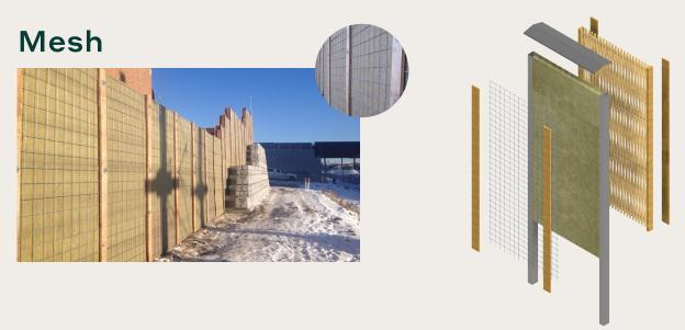
The mesh façade is a simple solution as well as a discrete and very affordable option. It is ideal when the façade is hidden or does not necessitate an important visual aesthetics.
