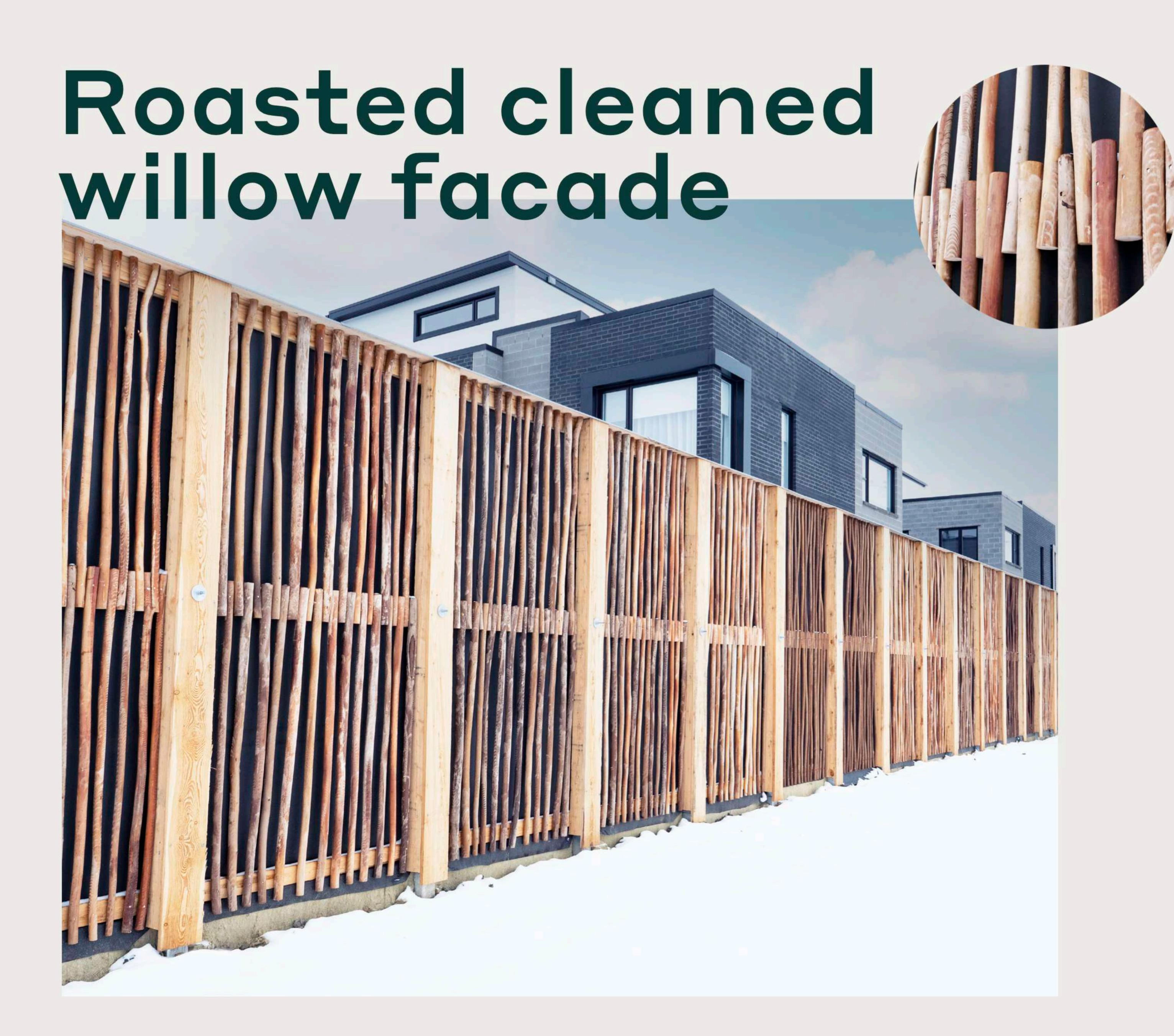
Roasted and debarked willow façade is made of larger diameter willow stems. The stems are interspersed which exposes the acoustic core of the sound barrier wall. This façade provides the natural aesthetic of willows at a reduced price.
