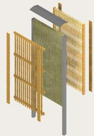
As efficient and easy to install, the larch façade is more traditional looking. It is made with larch laths that expose the rock wool core that provides sound absorption.
